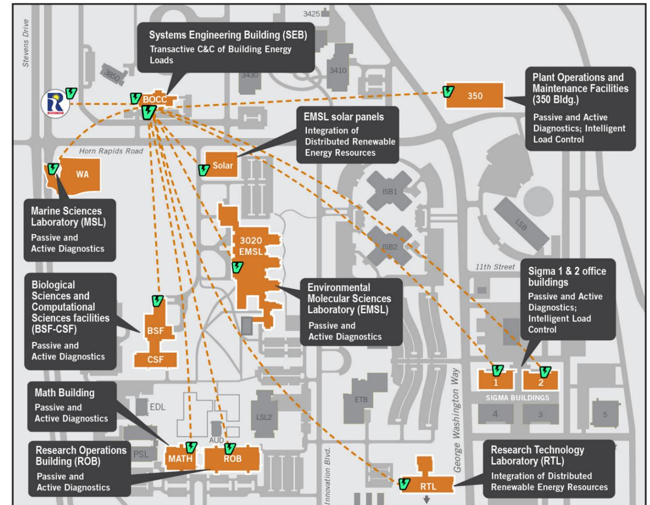
At PNNL, CETC experiments are occurring in a number of buildings. VOLTTRON™, represented by the green "v" icons, gathers building data and sends it to the Building Operations Control Center (BOCC), where campus building operations are monitored. The BOCC is located in the Systems Engineering Building.
