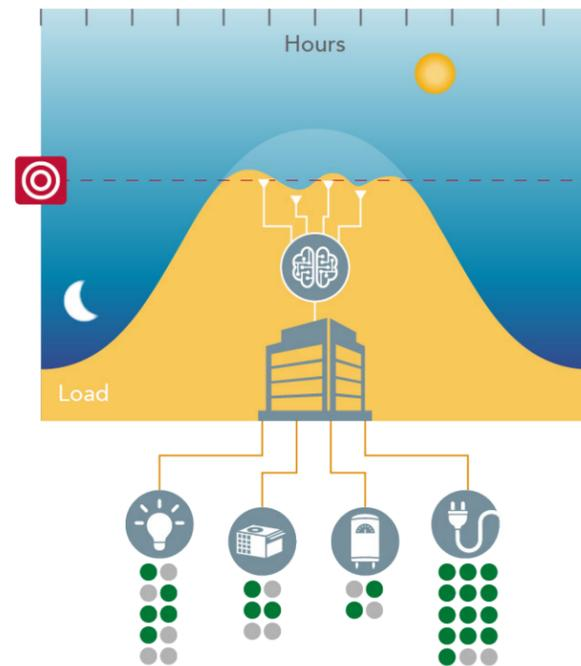
Intelligent Load Control is the "brain" behind coordination of building functions, such as lighting, heating and cooling, to adjust peak power loads and meet consumption targets. As illustrated in this graphic, ILC automatically prioritizes functions, turning them on (green dots) and off in a sequence that reduces power consumption, while concurrently making sure occupants remain comfortable.
